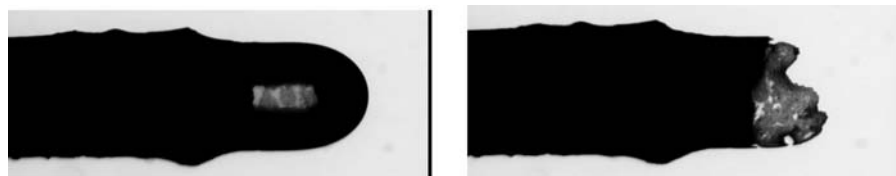
Figure 3. Image of the pendant drop of substance 2 at 282 K and 4.1 MPa.
